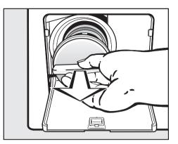
Unscrew the drain filter completely and then clean it thoroughly.
